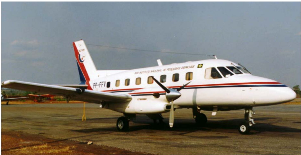
Figure 13. INPE Bandeirante aircraft instrumented for trace gases and aerosol measurements.
